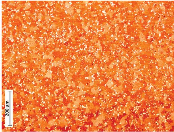
**Figure 12.** Microstructures after chemical etching of molybdenum powder with a high carbon content after sintering at 1900 °C under 70 MPa pressure for 30 min of holding.
