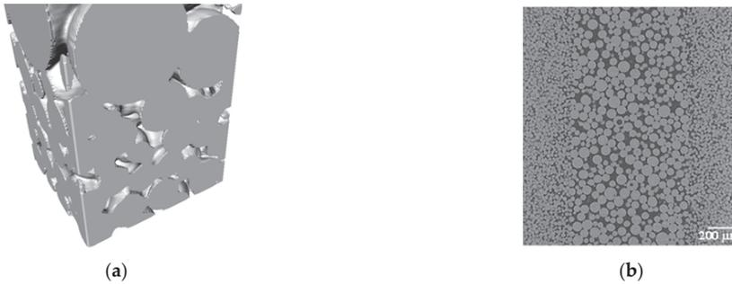
**Figure 5.** 3D and 2D virtual slices of samples of 1 and 2 mm in diameter, respectively, sintered at 1260 °C with a holding time of 5 min and a heating rate of 25 °C/min; (a) TBA-25 and (b) TBR-25.
