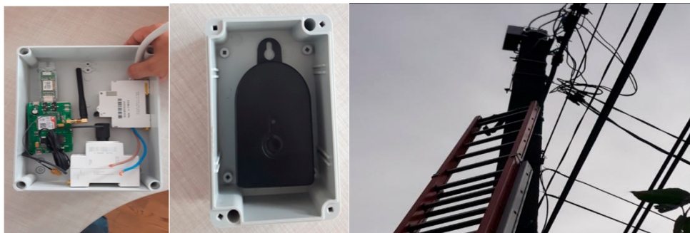
Figure 3. The pilot device assembly ( left ) and the mounting ( right ). The mounting was carried out by the beneficiary partner within the project.
