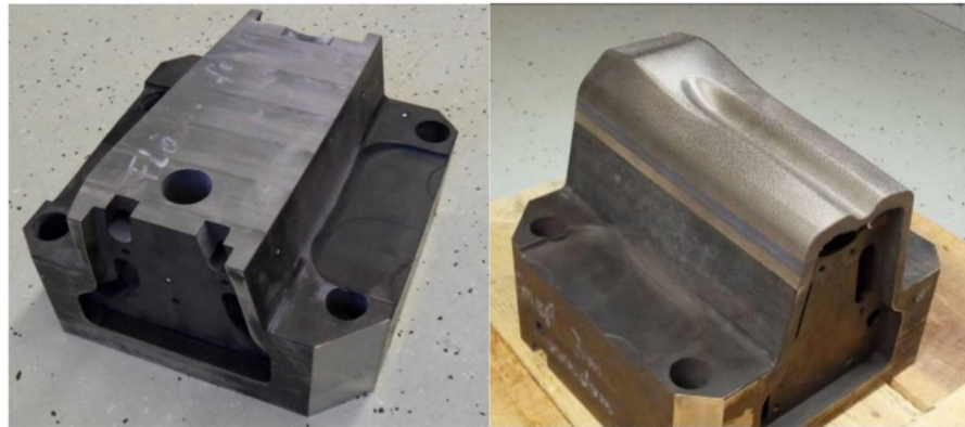
Figure 16. Tool insert for hot stamping made by the so-called hybrid tooling. The tool base was made by conventional milling of a conventionally made solid block ( left ). The functional structure including the optimized cooling channel was made by L-PBF in DIN 1.2709 over this tool base ( right ). The figure ( right ) shows the hybrid tool ready for final machining [133].
