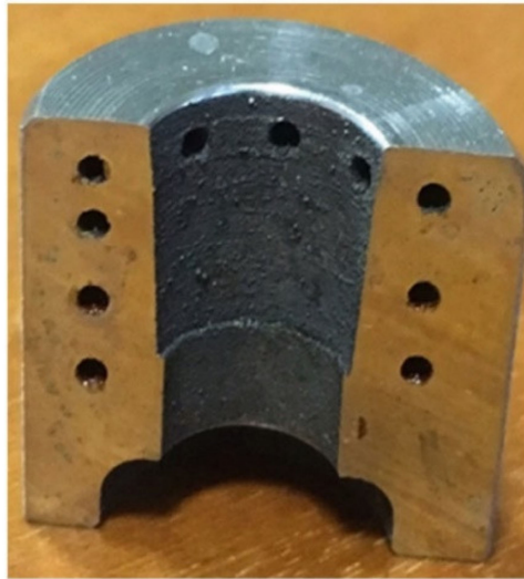
Figure 21. An extrusion die insert with conformal cooling channels through which liquid nitrogen flow. This die insert was made by L-PBF in H13 and integrated into a conventionally machined steel housing [134]. The height = 20 mm and the outer diameter = 25 mm [135].
