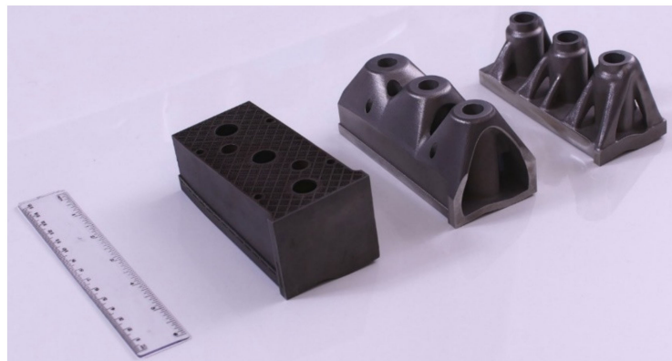
Figure 15. Three (3) versions of the industrial punch (Figure 13)—all 3D-printed (L-PBF) in DIN 1.2709: (left) with a honeycomb inner structure, (middle) after topology optimization using LS-TaSC and (right) after topology optimization using NX12 [62]. See also Figure 14.
