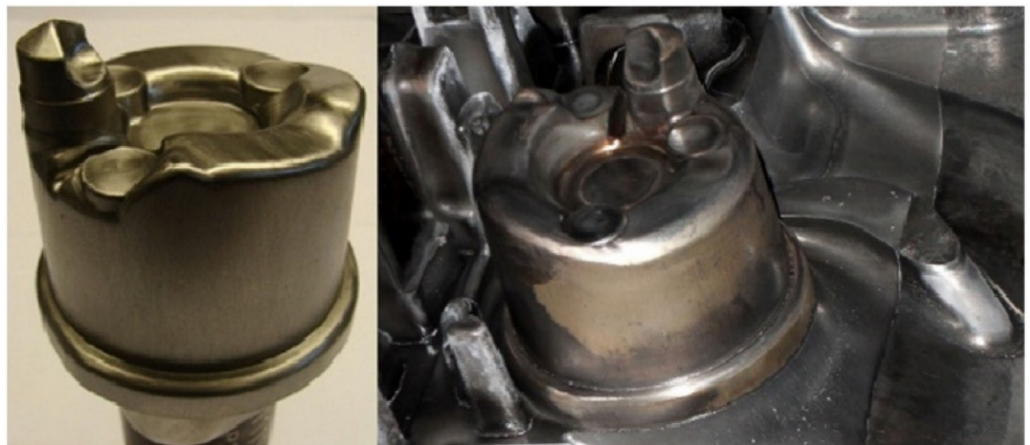
Figure 22. Aluminium die casting: (left) The tool insert was made in DIN 1.2709 by L-PBF, after which it was installed as a component in the die [133].
