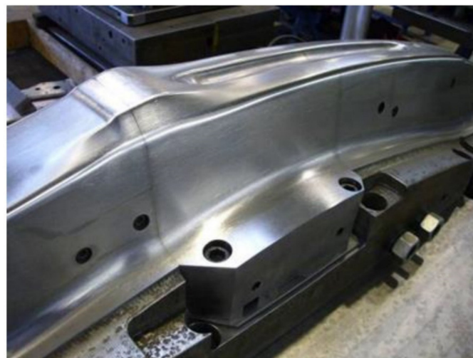
Figure 17. The assembled hot stamping punch [114].
