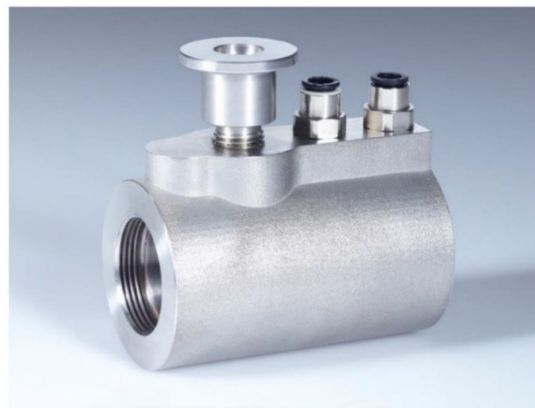
Figure 20. The calibration tool was made by L-PBF in 17-4PH [114].
