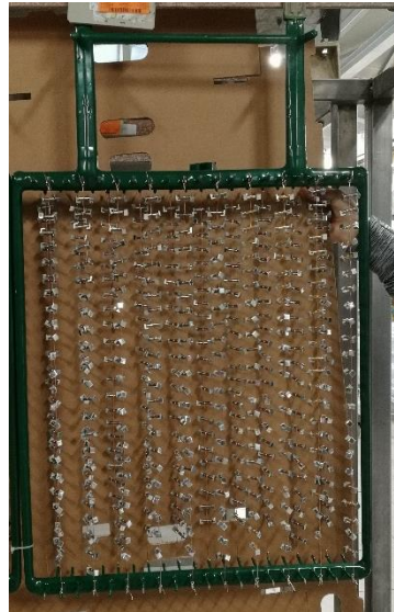
Figure 1. Typical galvanic frame.
