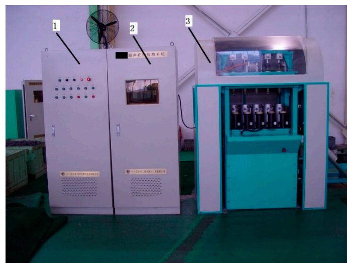
Figure 5. Appearance of testing equipment (1. PLC control unit; 2. PC control unit; 3. mechanical device).
