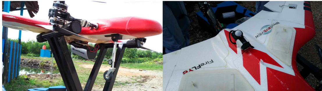
Figure 6. Firefly Pro 6 fixed-wing vertical takeoff and landing (VTOL) unmanned aerial system (UAS) carrying the multispectral sensor and the illumination sensor.
