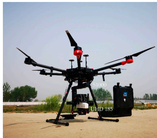
Figure 3. Unmanned aerial vehicle (UAV) hyperspectral imaging system.
