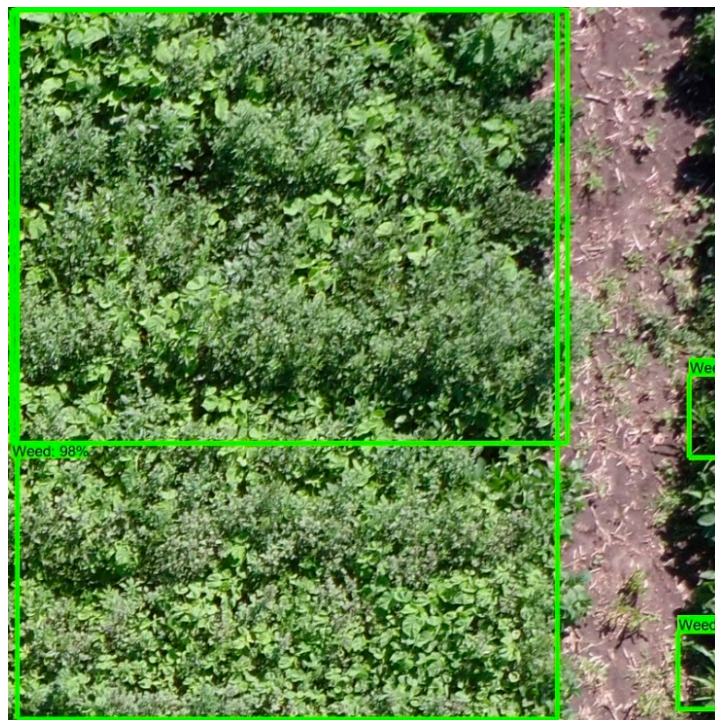
Figure 5. Example output image showing a weed patch annotated with single box in ground truth image detected as two boxes in output. This will lead to lesser precision as only the bigger box is considered true positive and therefore IoU is a better evaluation metric for this problem.
