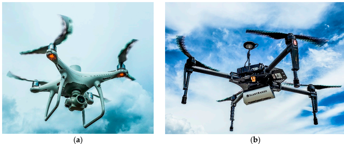
Figure 2. RGB and multispectral sensors used for data collection. (a) The DJI Phantom 4 Pro for RGB and (b) the DJI Matrice 100 platform with the SlantRange 3p sensor for multispectral data collection.
