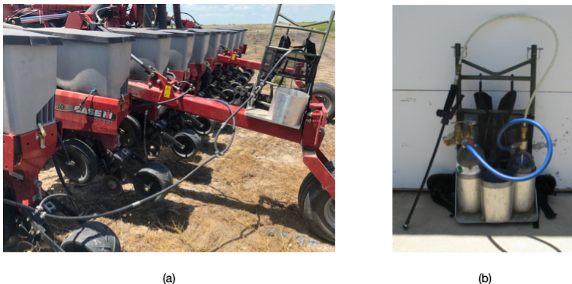
Figure 9. (a) A Case IH 1230 planter was used for in-furrow application; and (b) a CO 2 -pressurized backpack sprayer was used for manual treatments.
