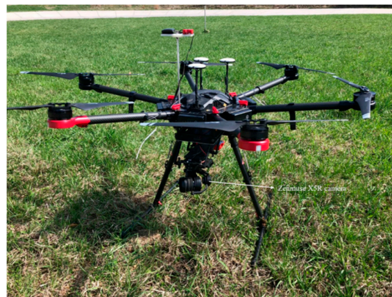
Figure 2. DJI Matrice 600 pro UAV platform with Zenmuse X5R camera.
