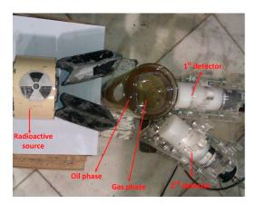
Figure 4. Experimental setup including 2 NaI detectors and one radioactive source [28].
