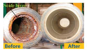
Figure 1. An oil pipeline before and after cleaning of the scale layer by chemical methods [26].
