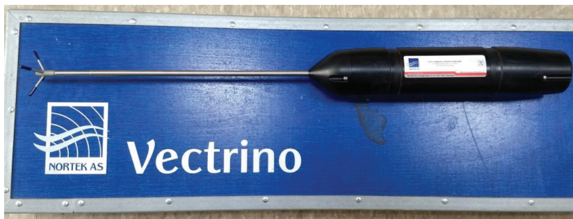
Figure 5. The acoustic Doppler velocimeter for the validation of the PIV-analyzed velocity field.
