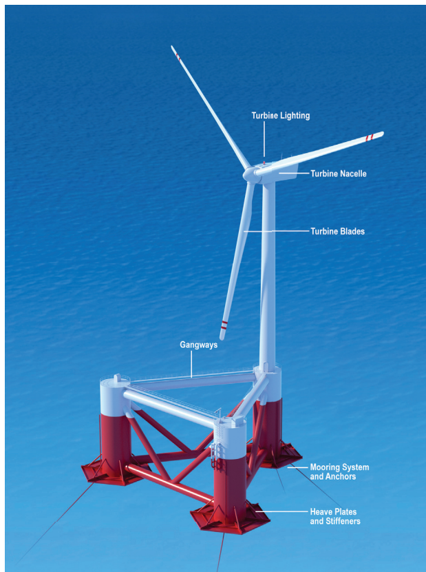
Figure 1. A floating offshore wind turbine showing heave plates attached to the structural columns [2]. Attributed to Untrakdrover/CC BY-SA ( https://creativecommons.org/licenses/by-sa/3.0 ).
