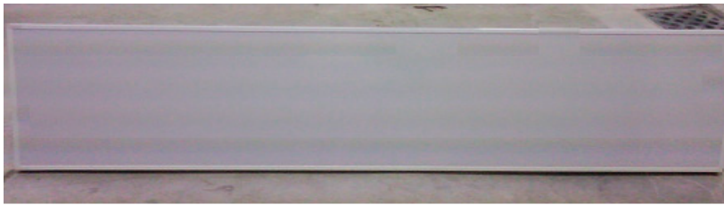
Figure 5. Rigid member (PVC): length 1.9 m; density 181.05 (kg/m 3 ); weight 8.6 kg, thickness 0.02 m.
