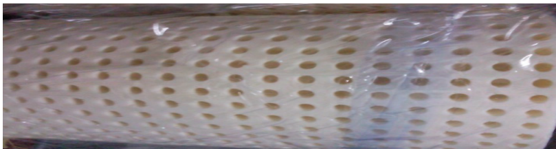
Figure 3. Latex component (Latex): length 1.9 m and 5.1 m; density 147.37 (kg/m 3 ); weight 7 kg, thickness 0.02 m.
