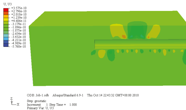
Figure 11. Vertical ground movement clouds of the initial state (m).
