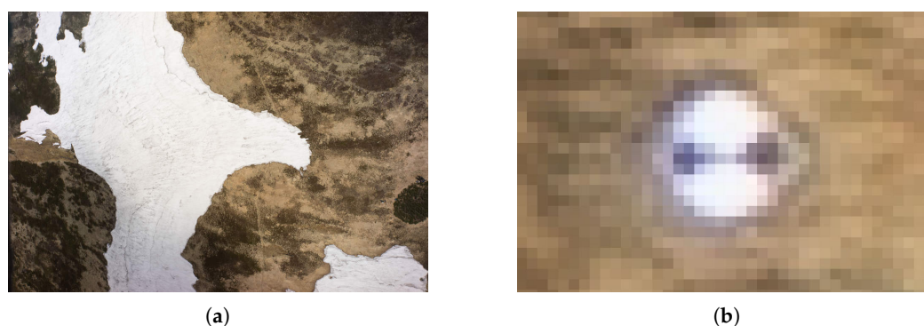
Figure 10. A photo captured from the height of 100 m AGL (a); a zoomed ground target (b).
