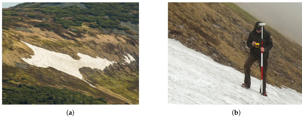
Figure 2. The isolated Mapa Republiky snow field during the spring season (a), and ground survey-based point determination of the snow field shape (b).
