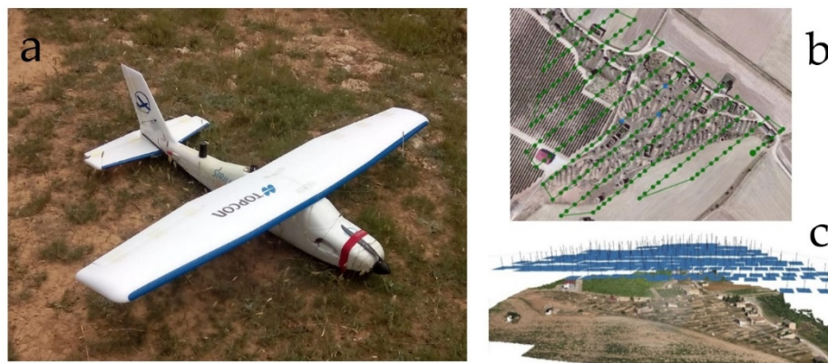
Figure 2. (a) Mavinci UAV used during the registration process. (b) Image orientation process task in Agisoft Photoscan® professional software ( http://www.agisoft.com/ ) showing flight paths and photocenters. (c) 3D view diagram of the recorded images.
