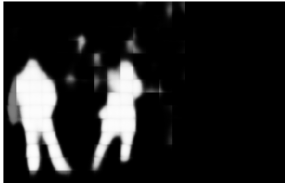
Figure 6. Image resultant of the combination of 64 \times 64 grayscale patches obtained by CNN predictions.
