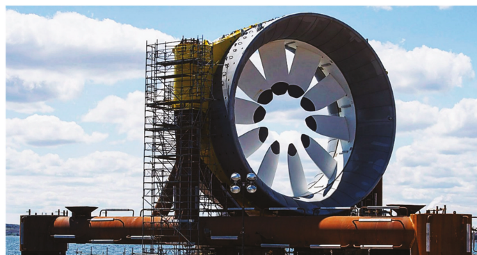
Figure 2. The 2 MW-rated OpenHydro ducted turbine. Adapted from [8], The Canadian Press/Andrew Vaughan, 2016.
