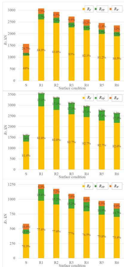
Figure 8. Decomposition of R_T for KCS (upper), KVLCC2 (middle) and BC (lower) for smooth and fouled surface condition.
