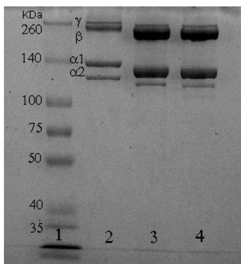
Figure 1. SDS-PAGE patterns of acid-soluble collagen (ASC) and pepsin-soluble collagen (PSC) from the red stingray skin. Lane 1: Standard protein marker (spectra multicolor broad range protein ladder); Lane 2: rat tail type I collagen; Lane 3: ASC collagen; Lane 4: PSC collagen.
