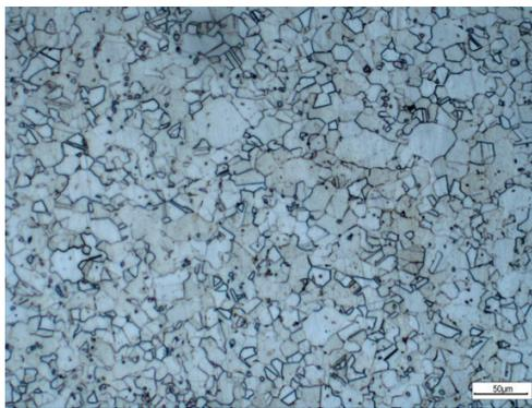
Figure 1. The original microstructure of the GH4169 forge piece.
