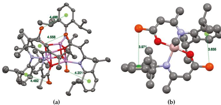
**Figure A3.** Orientation and distance of ketoiminate methyl carbon atoms (coloured orange) to aryl ring centroids (light green) of the *adjacent* ligands. Contrast the longer distances and poorer orientation in (a) **3b** with the more favourable situation in (b) the structure with the refcode BAMFAX (see [7]).
