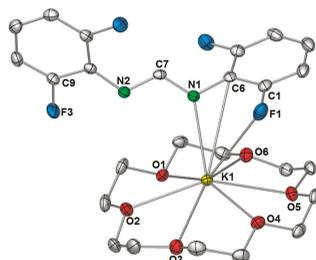
**Figure 6.** Molecular structure of  $[\text{K}(\text{DFForm})(18\text{-crown-6})]$  (**3**). Ellipsoids shown at 50% probability with hydrogen atoms omitted for clarity. Selected bond lengths (Å): K1–N1: 2.7994(12), K1–C6: 3.4836(14), K1–C1(non-bonding): 3.6886(15), K1–F1: 3.2809(11), K1–N2(non-bonding): 3.9843(13), K1–O(crown): range: 2.8255(11)–2.9525(11), average: 2.89. C1–F1: 1.3584(18), C1–C6:1.401(2), C9–F3: 1.3576(16), C7–N1: 1.3224(18), C7–N2: 1.3161(18).
