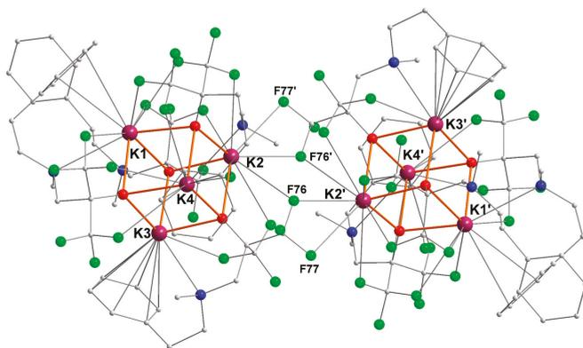
**Figure 1.** Representation of the molecular solid-state structure of the potassium–arene complex  $[(RO^1)K]_4$  ( $[1]_4$ ). Color code: purple, K; green, F; blue, N; red, O; grey, C. H atoms omitted for clarity.
