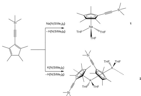
**Scheme 2.** Synthesis of  $[\text{NaCpMe}_4(\text{C}\equiv\text{CSiMe}_3)(\text{THF})_3]$  and  $[\text{KCpMe}_4(\text{C}\equiv\text{CSiMe}_3)(\text{THF})_2]_n$ .
