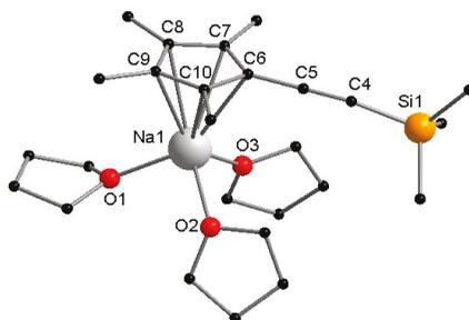
**Figure 1.** Molecular structure of **1** in the solid state. Hydrogen atoms are omitted for clarity. Selected bond lengths [Å] and angles [°]: Na1–C6 2.691(4), Na1–C7 2.673(4), Na1–C8 2.672(4), Na1–C9 2.717(4), Na1–C10 2.736(4), C4–C5 1.223(6), Na1–O1 2.289(3), Na1–O2 2.321(3), Na1–O3 2.293(3), O1–Na1–O2 96.70(2), O2–Na1–O3 95.75(12), O3–Na1–O1 96.14(12).
