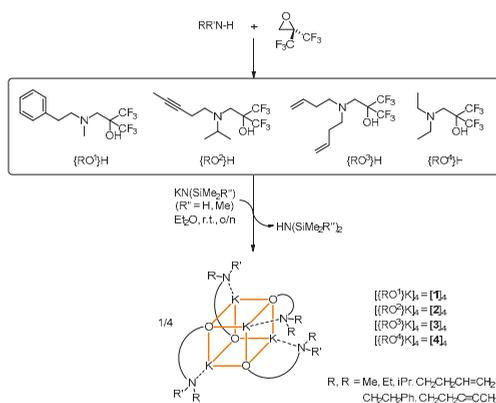
**Scheme 1.** Fluoroalcohols used in this study, with a synthetic scheme for the preparation of the tetranuclear potassium fluoroalkoxides [(RO<sup>x</sup>)K] [1]<sub>4</sub>–[4]<sub>4</sub>. A representation of the cuboid structures of these complexes is given; K<sup>+</sup>...F and K<sup>+</sup>...C $\pi$  secondary interactions not displayed.
