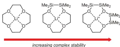
**Scheme 1.** Binding modes and relative binding affinities of Li<sup>+</sup> in [12]crown-4, 1,2-disila[12]crown-4, and 1,2,4,5-tetrasila[12]crown-4.
