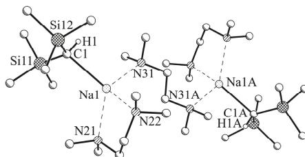
**Figure 6.** Molecular structure of  $[\text{NaCH}(\text{SiMe}_3)_2]_2\text{-3TMEDA}$ , **2b**. Selected hydrogen atoms and disordered units of minor occupancy are omitted for clarity. Symmetry operator A:  $-x+1, -y+1, -z+2$ .
