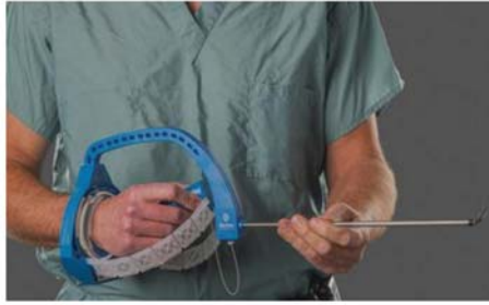
Figure 9. The FlexDex laparoscopic needle driver offers wristed instrumentation similar to DaVinci robotic instruments without the costs of the robot, but still more expensive than conventional laparoscopic instruments. Image taken from https://flexdex.com [99].
