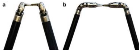
Figure 6. Comparison of the DaVinci 8 mm (a) and 5 mm diameter instruments (b). Due to their tentacle-like continuum tool shafts, the smaller diameter instruments need more operative space than the 8 mm instruments and are therefore not suitable in smaller cavities, such as infants. Figure taken from Marcus 2015 [62].
