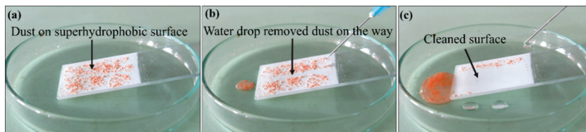
Figure 5. Self-cleaning performance of the prepared superhydrophobic AD-2 coating. (a) Dust particles on the superhydrophobic coating, (b) water drops carrying the dust particles, and (c) the cleaned surface.
