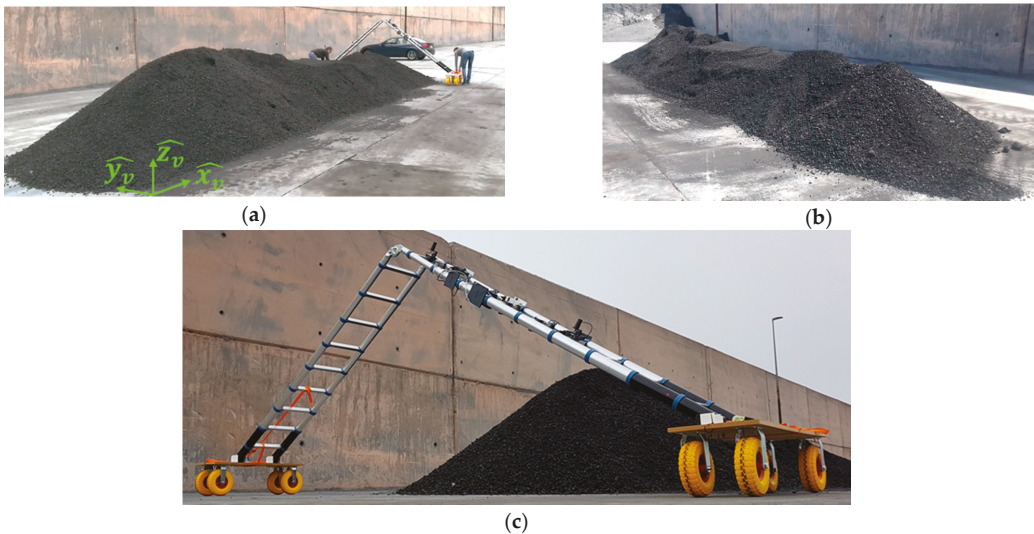
Figure 7. (a,b) Scaled stockpile from two different perspectives; (c) the ladder with the sensors prior to conducting the stockpile scanning.
