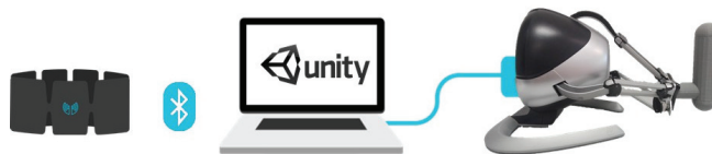
Figure 1. Scheduled illustration of the upper limb rehabilitation platform: Myo Gesture armband (left object in image) and Novint Falcon device (right object in image).
