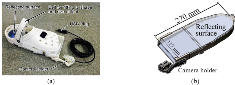
Figure 1. Overview of the system: (a) photo of the clog-integrated plantar visualization system and (b) dimensions of the underpart of the plantar observation system.
