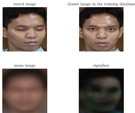
Figure 6. Test image, closest image, mean image and eigenface.
