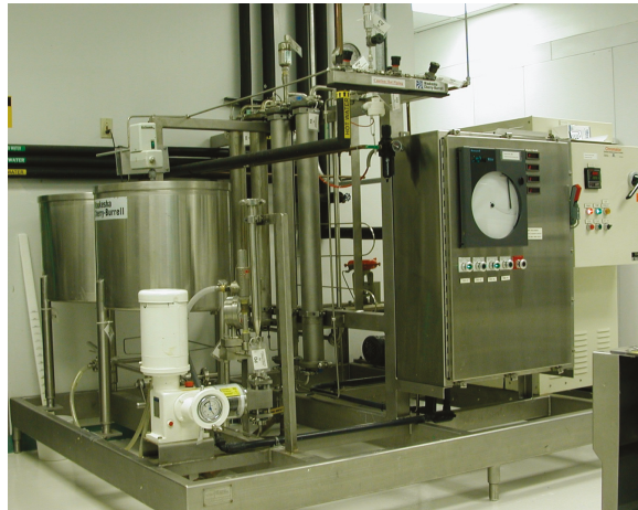
Figure 1. Frontier Scientific’s flash sterilization system used for the processing of insect media. From left to right: diet tank, pump, processing tubes, coiled spiralthermes, and control station.
