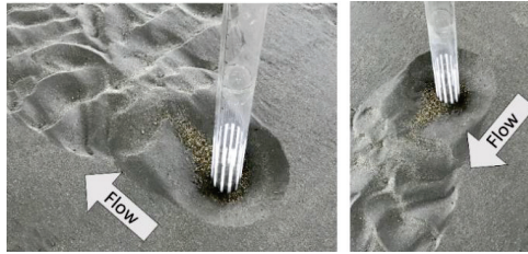
Figure 8. The scour hole in the approximate equilibrium condition.
