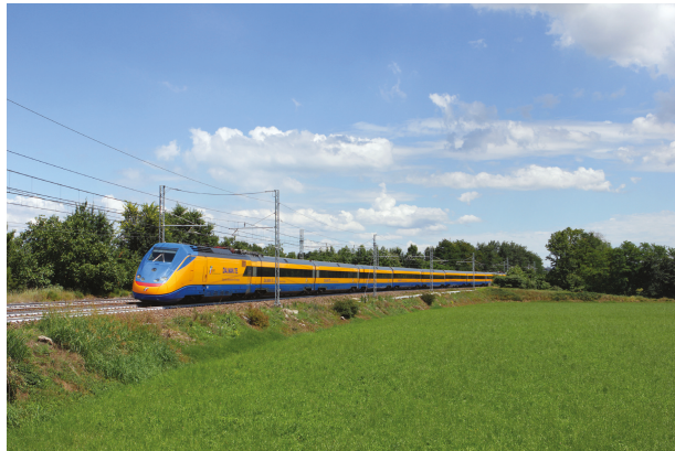
Figure 8. ETR.500 Y 2 “Dia.man.te”, high speed (300 km/h) visual inspection EMU (courtesy of © Stefano Paolini).
