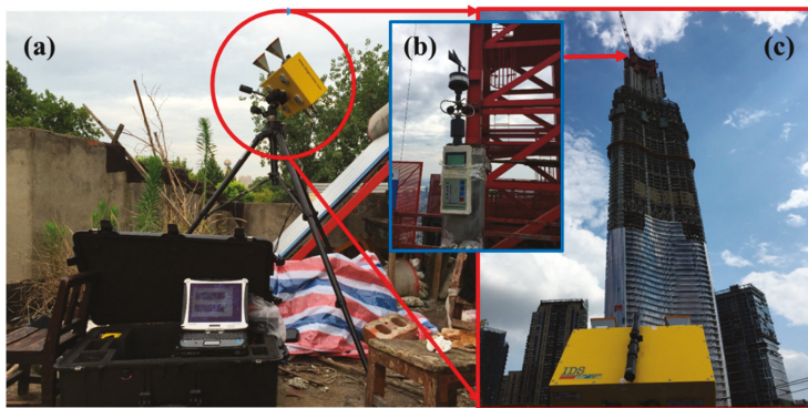
Figure 4. Location of the IBIS-S-1 system in the north–south direction. (a) View of the IBIS-S-1 interferometric radar on S1 (located in a farmhouse roof). (b) Weather station installed on the roof of the monitored building. (c) Ground view of the WGC from the location of the IBIS-S-1 interferometric radar.
