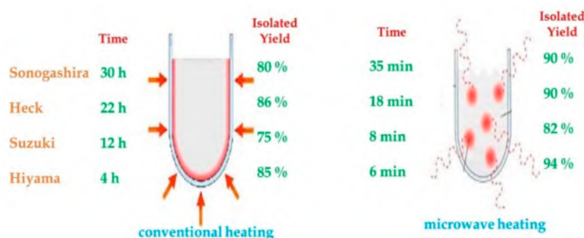
Figure 1. A comparison of time and yield for standard protocols of various coupling reactions. Reproduced with the permission of reference [28], Copyright 2016 Elsevier B.V.
