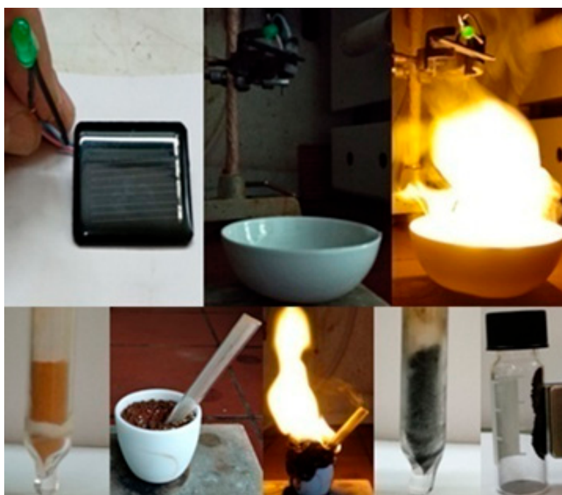
Figure 5. Top: ignition of the coffee- \text{Na}_2\text{O}_2 mixture generates enough thermal radiation and light to turn on a miniature silicon photovoltaic device. Bottom: the ignitable mixture served as a heat source for the in-situ thermal transformation of ferric acetate (orange powder at far-left) into magnetic iron oxide (black solid at far-right). For this purpose, a small quartz tube was charged with the precursor and then merely dipped into the ignition mixture. Notice the release of smoke from the top rim of the tube due to thermal decomposition of ferric acetate.
