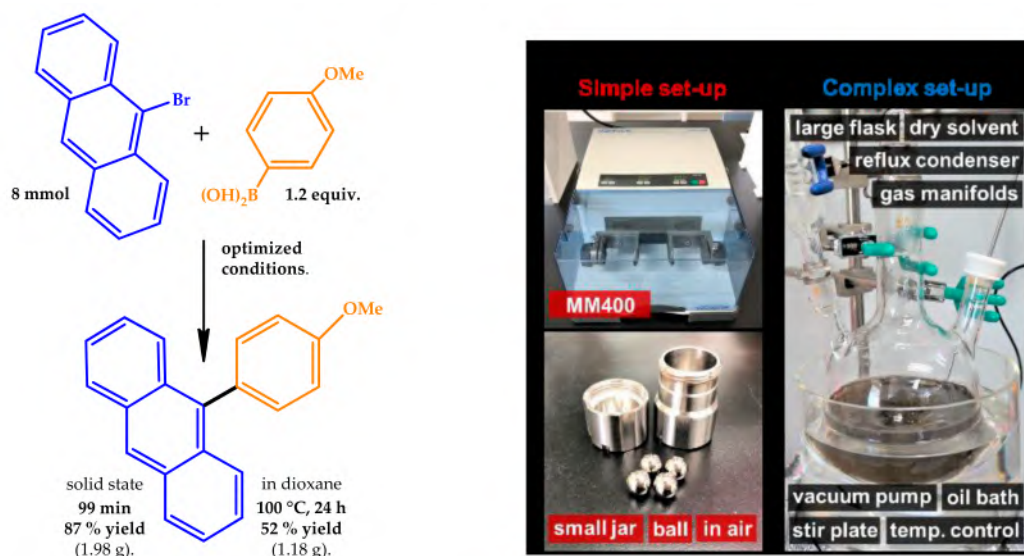
Figure 4. (Left): Reaction scheme for the solid-state cross-coupling of 9-bromoanthracene with p -methoxyboronic acid. (Right): Solid-state coupling reaction on the gram scale. Reproduced with the permission of reference [47], Copyright 2019 Royal Society of Chemistry.
