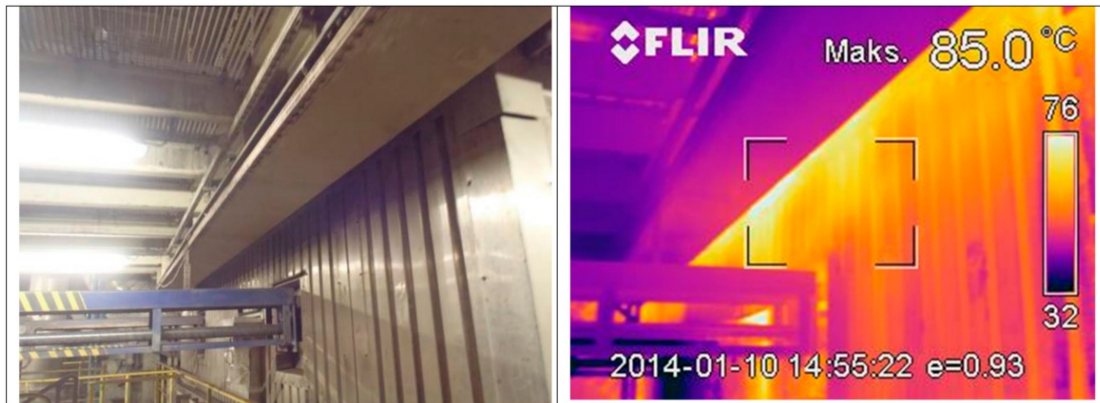
Figure 8. Temperature distribution at the soot blower entrance point into the furnace chamber.
