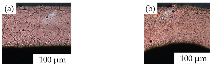
Figure 27. Microstructure of the wrinkled tube obtained from the cylinder-shape warm THF in Stage (2) at 250 °C: (a) microstructure in the non-deformed area; (b) microstructure at the top of the wrinkle.
