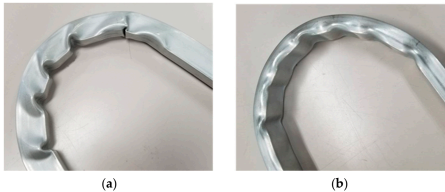
Figure 10. Result of rotary draw bending (Without a mandrel and axial tension); (a) Folding ( H_0 = 20 , R = 50 ); (b) Wrinkling ( H_0 = 10 , R = 50 ).
