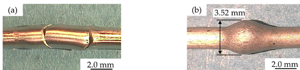
Figure 7. Expansion behavior of the tube at R.T and 250 °C: (a) fractured tube at R.T; (b) expanded tube at 250 °C.
