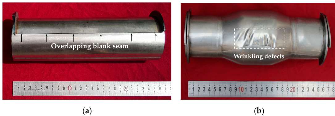
Figure 13. Hydroforming of overlapping blank under axial constraints in experiment results. (a) Initial blank; (b) hydroformed part.
