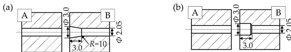
Figure 9. Geometry and dimensions of the tube hydroforming dies used in this study: (a) a taper-cavity die; (b) a cylinder-cavity die.
