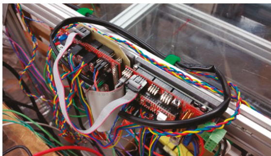
Figure 6. Assembled two RAMPS 1.4 with custom I/O PCB per the KiCAD-PcbNew specification.
