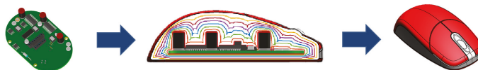
Figure 3. Build-object defined as a 3D CAD model of a populated circuit board (left) and desired surface defined as 3D CAD model of a computer mouse. A cross-section of equipotential curves derived from solutions to (2) equation between the build-object and desired surface is shown in the center.
