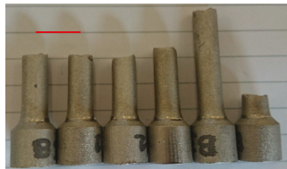
Figure 6. Set B (175 W) specimen fracture locations.
