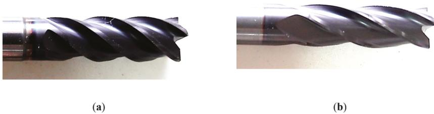
**Figure 1.** Ceramic-coated tungsten carbide side- and end-mill cutters having helix angles of (a) 42° and (b) 30°.
