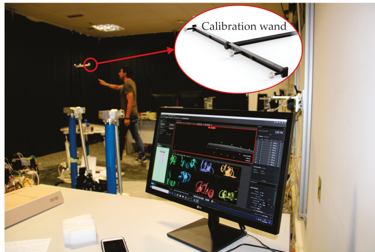
Figure 6. Calibration wand and experiment to determine the location of the markers.
