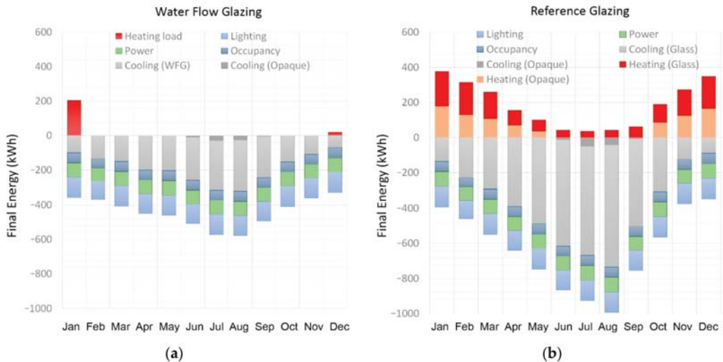
Figure 7. Estimation of final electric energy consumption of the prototypes: (a) Water Flow Glazing prototype with a water-to-water heat pump; (b) Reference glazing prototype with an air-to-air heat pump.
