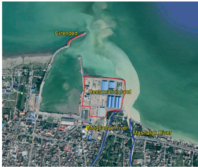
Figure 3. Changes in Nowshahr port layout since the year 1989 until now. Commission year: Initial layout in 1939, main breakwater extension in 1996, and reclamation land in 2012.
