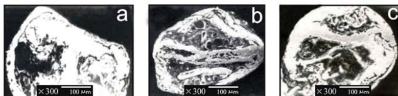
Figure 13. Cross-sections of various forms of hollow gold from natural: (a) internal partition; (b) filamentous twisted gold; (c) shell.
