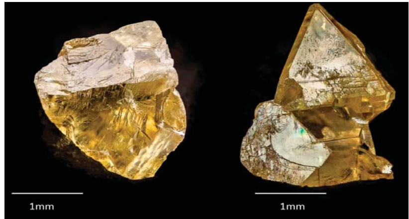
Figure 33. Microphotos of the synthetic sphalerite crystals with admixtures of Ag and In, synthesised using the gas transport method (sample 4197). According to EPMA [108], C_{Ag} = 4.74 \pm 0.82 wt%, C_{In} = 5.15 \pm 0.46 wt%. However, according to (N. Trofimov, pers. com.), C_{Ag(min)} = 3.41 wt%; C_{Ag(max)} = 75.99 wt%, because of the capture of the tiny Ag_2S inclusions in the analysis, and C_{In(min)} = 0.64 wt%, C_{In(max)} = 5.85 wt%.
