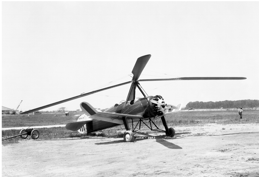
Figure 1. The picture above (public domain) shows a PCA-2 autogiro built in the United States by Pitcairn under license of the Cierva Company. This unit was used by the National Advisory Committee for Aeronautics (NACA) for research purposes on rotor systems (c.f. [2]).
