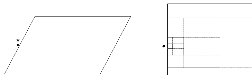
Figure 3. The partition method in Case II (left: location of the singular point z^* and projection point z . right: the nonuniform grid).
