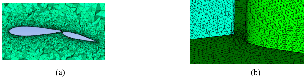
Figure 6. The encrypted mesh in (a) mid-span and (b) bottom wall of the slot.
