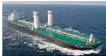
Figure 1. "Kaili" VLCC with wingsail.
