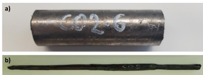
Figure 1. (a) Ingot cast in the levitation vacuum furnace and (b) bar forged from the ingot.
