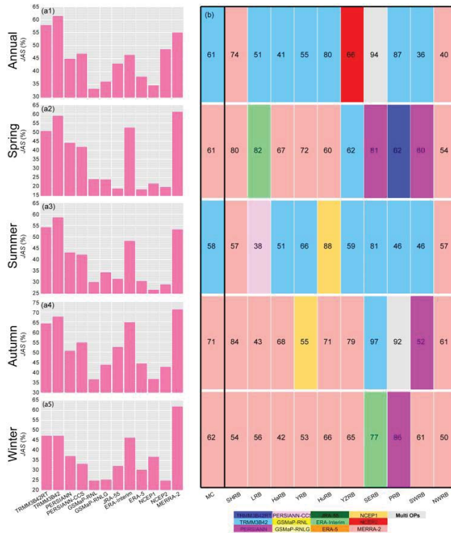
Figure 8. MC joint AS (JAS) values derived from the selected 12 precipitation products (a1–a5), and JAS-based optimal products (OPs) for MC and ten WRRs (b). For figures (a1–a5), JAS is computed with Equation (6), indicating the capacity of a given product to rightly detect the signs of both P_d and P_n changes relative to the observed data. In (b), the number in each box represents JAS values (%) of the OP, which has been labelled with different colors.
