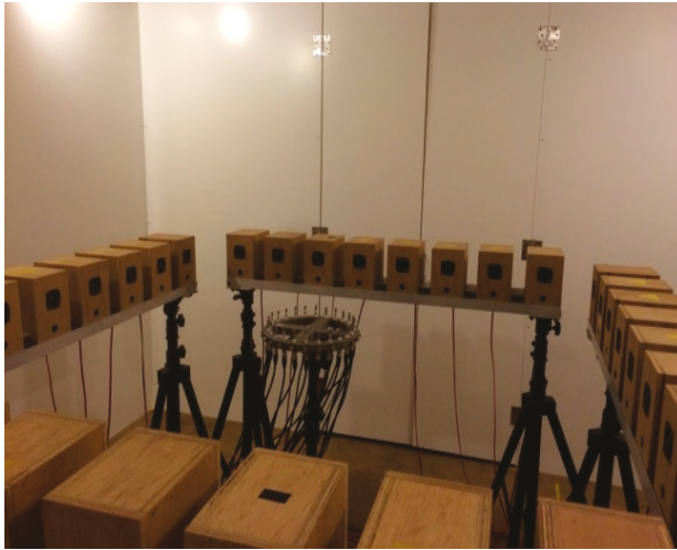
Figure 11. Sound field synthesis experimental arrangement in a 3.6\text{ m} \times 3.6\text{ m} \times 2\text{ m} live room fitted with reflective walls.
