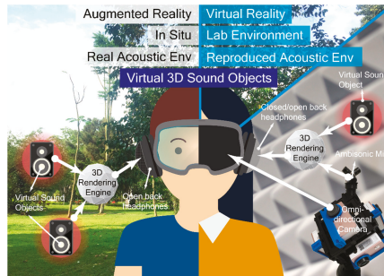
Figure 8. (Left) AR setup with spatial audio from rendered virtual sound objects for in situ environments. (Right) A lab-based VR setup from omni-directional camera recordings and a reproduced acoustic environment using spatial audio from ambisonic microphone recordings and rendered virtual sound objects [97].
