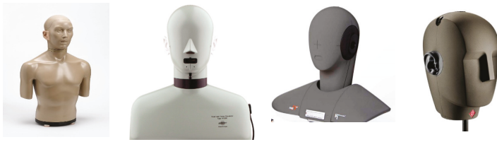
Figure 4. Dummy heads (from left to right): KEMAR, Brüel & Kjær 4128 HATS, Head Acoustics HMS III, and Neumann KU-100. Note that Neumann KU-100 dummy head is torso-free.
