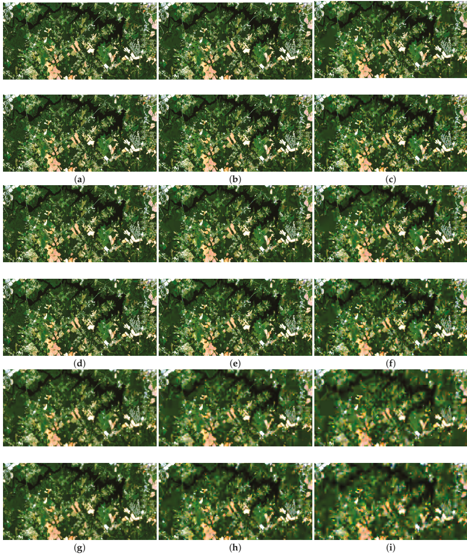
Figure 8. Visual comparison of HEVC and JPEG 2000 at the same level of PSNR. The first column corresponds to Sentinel 2 images of 10, 20, and 60 m generated at high PSNR of 70 [dB]. In the second column are images with 60 [dB], while in the last column are images with approximate lower borderline quality of 56 [dB]. Each pair of rows (3 in total) represents satellite images at exclusively one of the following spatial resolutions: 10 m (a–c), 20 m (d–f), and 60 m (g–i), respectively. The first row in each pair corresponds to obtained HEVC results, e.g., the first row of (a–c), while the second row in each pair is reserved for JPEG 2000 results with the same level of PSNR and spatial resolution (e.g., 10 m for (a–c)). Presented image detail was taken from the test scene N o 7 in Table 1, Figure 2g.
