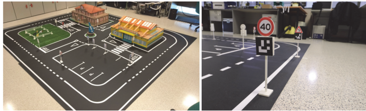
Figure 1. Left: A general overview of the real Robobo SmartCity layout. Right: A snapshot of two different traffic signs with an ArUco marker.
