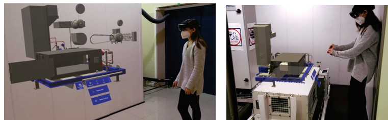
Figure 2. Expanded view of the parts of the digital twin of the cooler (left) and user performing a repair procedure on the real cooler, being guided by the developed AR application (right).
