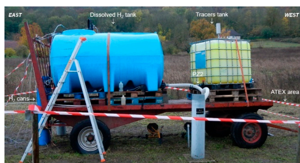
Figure 5. View of the injection device.
