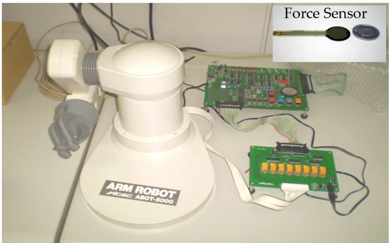
Figure 8. 4-DoFarm robot used to learn force and joint velocity control techniques.
