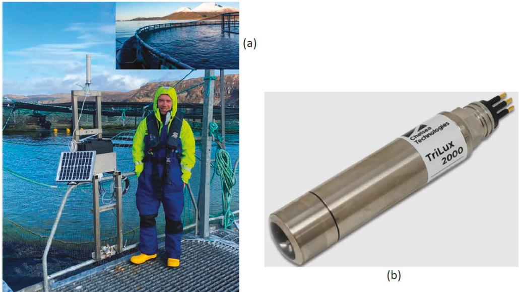
**Figure 1.** (a) Installation site of the TriLux multiparameter fluorometer at the salmon aquafarm, with the inset image depicting the larger part of the salmon cage; (b) Chelsea Technologies' TriLux multiparameter fluorometer which monitors three key algal parameters in a single probe [15].
