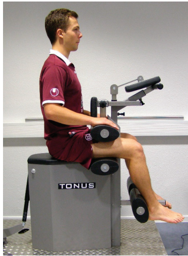
Figure 3. Measurement of the isometric torques of the hamstrings (pelvic fixation not shown).
