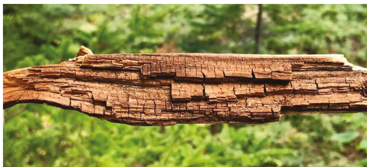
Figure 1. Classic advanced brown rot fungal decay in a softwood. Note the checks (cracks) which cut across the grain of the wood giving the wood a cubical appearance. In early stages of brown rot decay, the wood can appear unchanged from undecayed wood, yet significant mechanical property loss may be sustained even in early brown rot decay stages.
