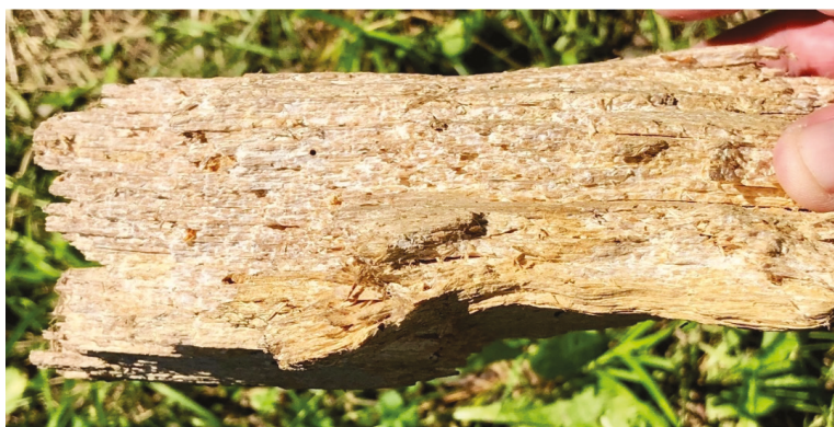
Figure 2. Advanced stage of white rot simultaneous decay. The wood in this advanced state of decay can be quite spongy and lightweight when dried. However, when decay is active, the wood will be moist and stands of wood can often be peeled from the surface along the grain. The flecks of white in the image are mycelial mats of the fungus.
