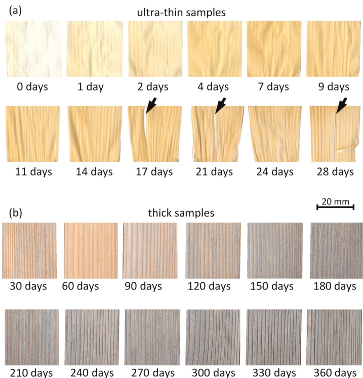
Figure 2. Appearance changes of ultra-thin (a) and reference thick (b) wood samples exposed to natural weathering in San Michele All'Adige (Italy). Note: arrow indicate weathering-induced damages to wood cells.
