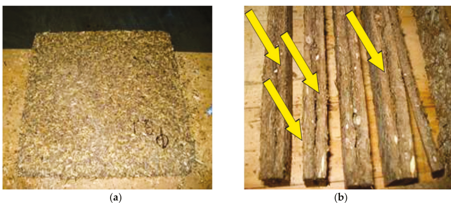
Figure 4. Cracks (blows) in the core layer of boards made with 50% PO leaves, (a) after hot pressing; (b) after trimming.
