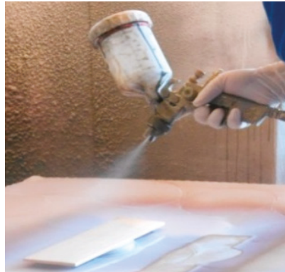
Figure 3. Application with the spray gun.
