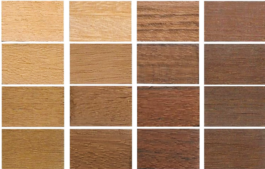
Figure 1. Visual comparison of contrast among the exposed and non-exposed surface (from left: garapa, tatajuba, courbaril and massaranduba; from top: fresh wood, after 24 h of UV irradiation, after 1 cycle of artificial weathering, after 4 cycles of artificial weathering).
