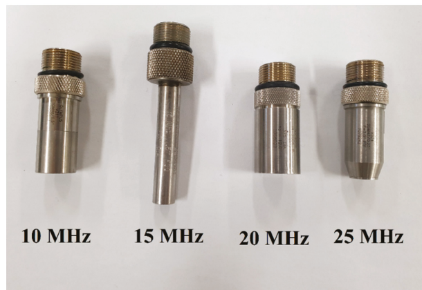
Figure 10. Transducer probes with each different frequency band used to measure the echo signals.
