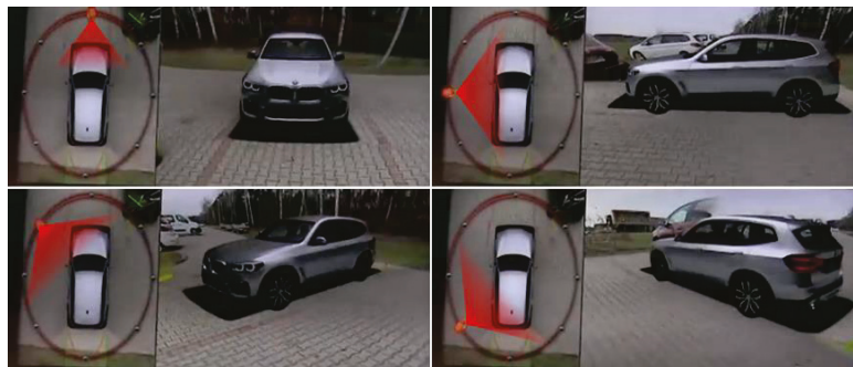
Figure 6. Reconstructed AVM images according to the properties of the virtual AVM camera.
