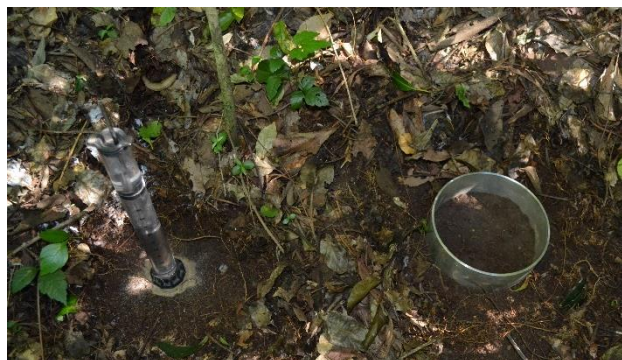
Figure 1. Picture in the forest site showing the mini-disk infiltrometer and the steel ring used for the Beerkan infiltration test.
