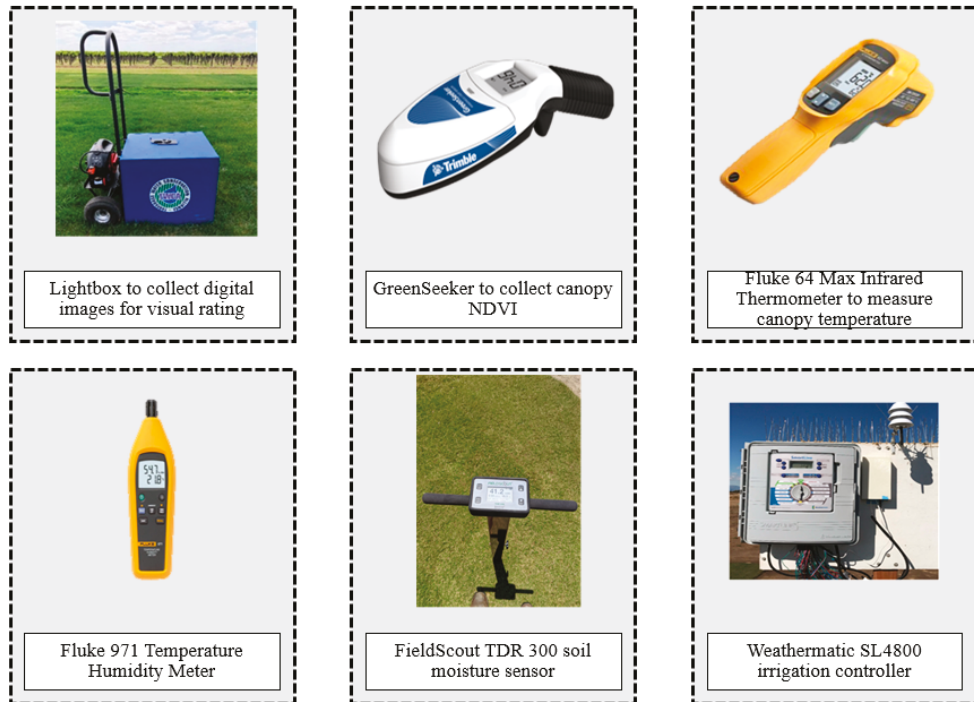
Figure 3. An overview of the sensors and tools used in this study and the companion paper [23].
