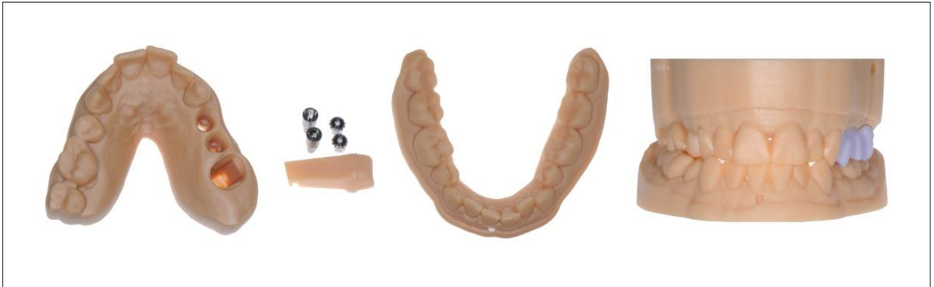
Figure 6. Additive manufactured models for implantology.
