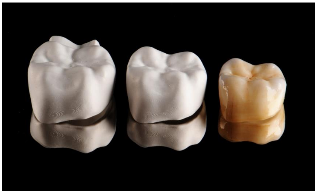
Figure 18. 3D printed Zirconia crown in the green and the white state and finally sintered.
