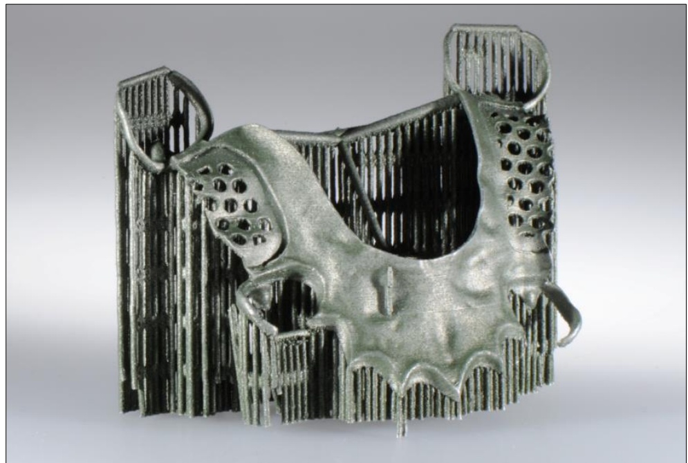
Figure 4. Laser sintered removable partial denture with support structures.
