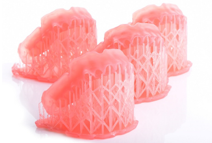
Figure 2. Exemplary 3D printed denture bases (here: stereolithography (SLA) with 45° build angle).
