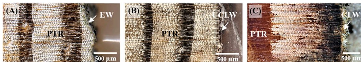
Figure 3. Stereoscopic observation of the outermost annual ring. (A) Earlywood (EW); (B) uncompleted latewood (UCLW); (C) completed latewood (CLW); PTR: previous annual ring.
