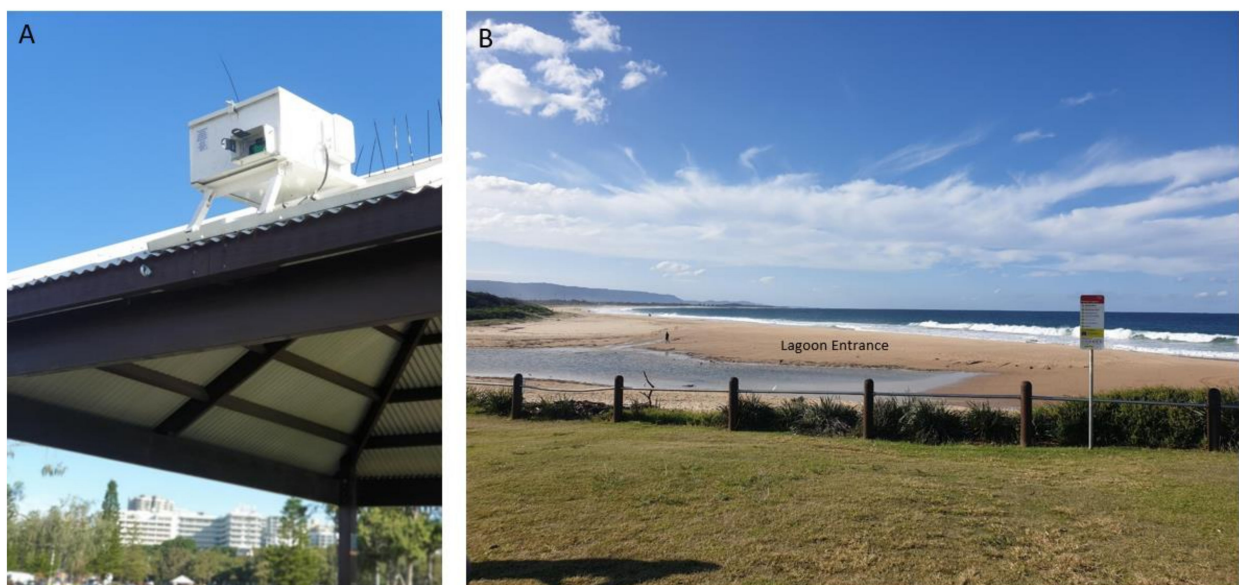
Figure 4. (A) Remote monitoring station; (B) Field of View from Lidar Sensor.
