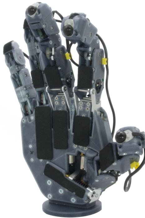
**Figure 1.** PUT-Hand—An open source dexterous robotic hand.
